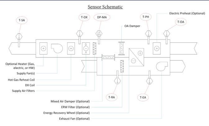
All sensors included with your unit for field installation must be installed prior to start-up or the unit will not operate properly. Sensors are typically either NTC, 4-20mA, or 0-5 VDC.
