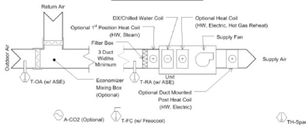
All sensors included with your unit must be installed prior to start-up or the unit will not operate. Sensors are typically either NTC type, 4-20mA, or 0-5 VDC.
