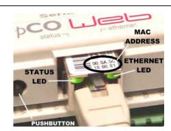
Figure 1.b - MAC address and indicator LEDs
