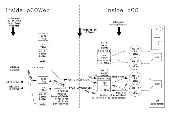
Figure C.a - Communication between **pCOWeb** - **pCO** atoms
