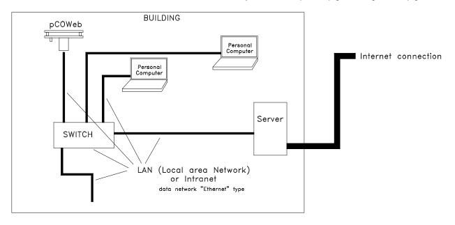
Figure 1.a - **pCOWeb**: example of network connection
