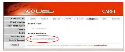
Figure 9.n – Plugin page: **pCOWeb** has found one or more Plugins to be installed
