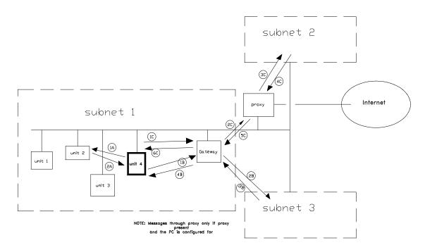
Figure B.a - Communication in a network
