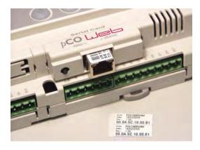
Figure 2.d – Securing **pCOWeb** with the cover
