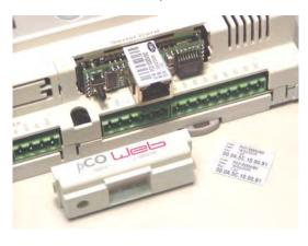
Figure 2.c – Inserting **pCOWeb** in the **pCO** controller
