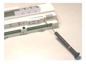
Figure 2.b – Removing the cover from the **pCO** controller
