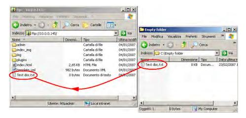
Figure 4.j – Using Windows Explorer as the FTP client
