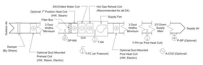
All sensors included with your unit must be installed prior to start-up or the unit will not operate. Sensors are typically either NTC type, 4-20mA, or 0-5 VDC.
