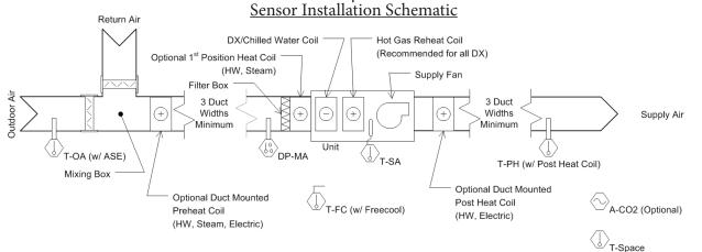
All sensors included with your unit must be installed prior to start-up or the unit will not operate. Sensors are typically either NTC type, 4-20mA, or 0-5 VDC.
