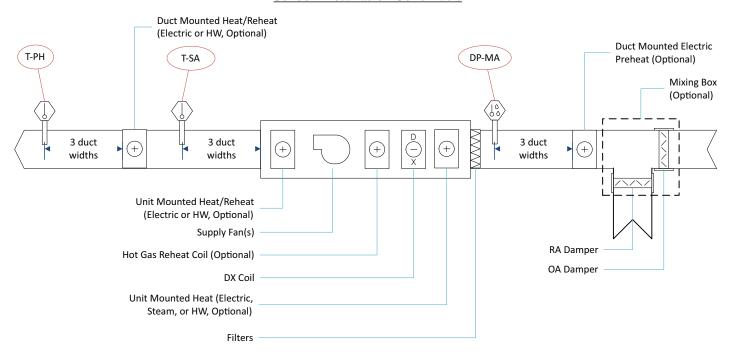
All sensors included with your unit must be installed prior to start-up or the unit will not operate. Sensors are typically either NTC type, 4-20mA, or 0-5 VDC.
