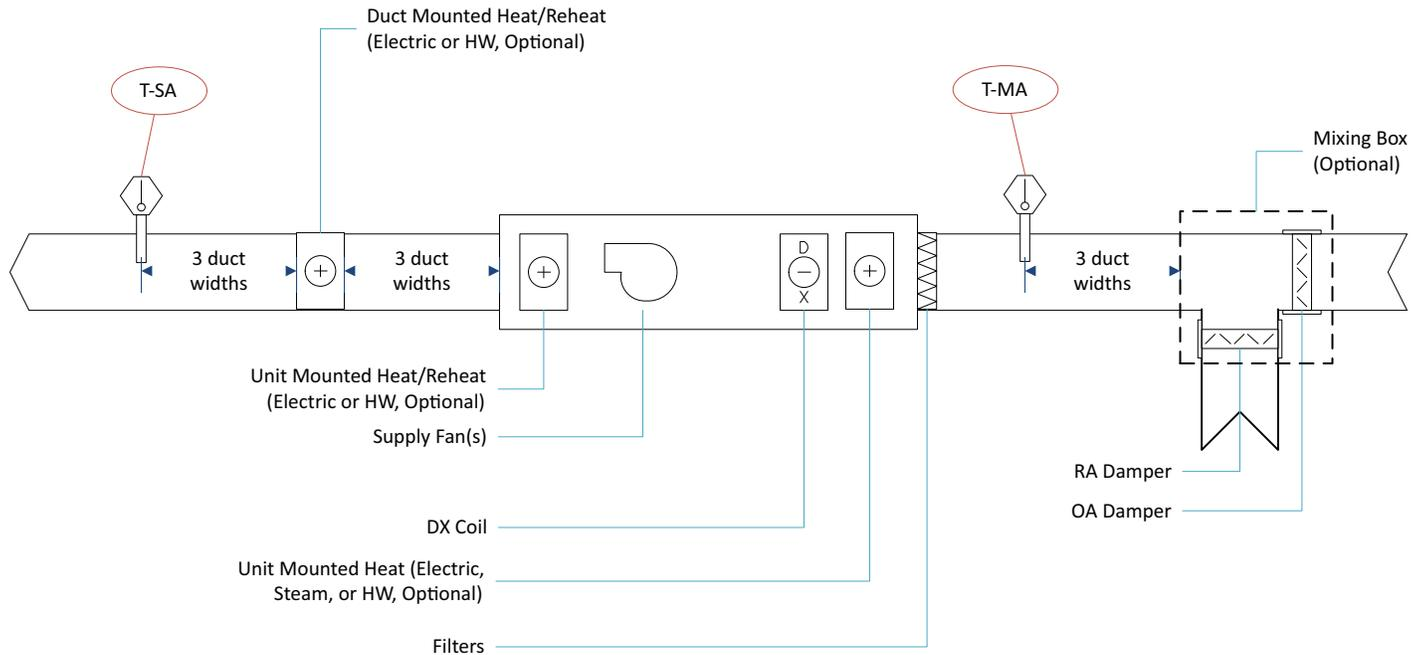
All sensors included with your unit must be installed prior to start-up or the unit will not operate. Sensors are typically either NTC type, 4-20mA, or 0-5 VDC.
